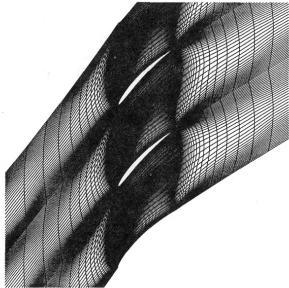
Fig. 2 H-mesh used for the NPHASE, steady and unsteady, inviscid, transonic simulations
