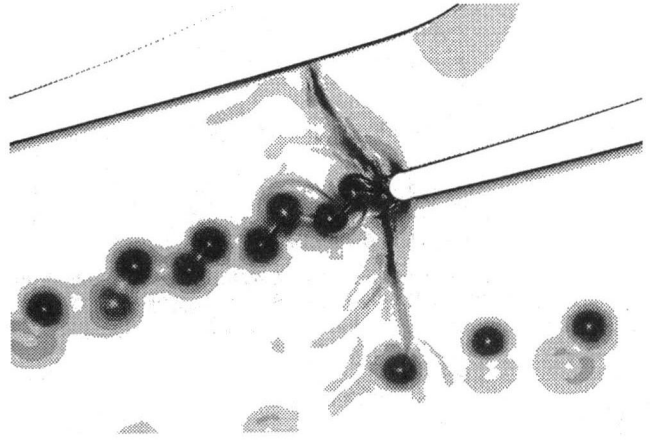
Fig. 7 Numerical schlieren of vortex street at M_2 = 1.0 after \sim 100 periods
