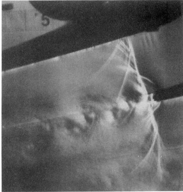
Fig. 8 Experimental schlieren of vortex street at M_2 = 1.0
