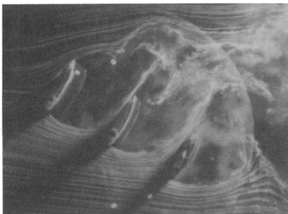
Fig. 4 Smoke-wire flow visualization of baseline strut: \alpha = 60 deg
